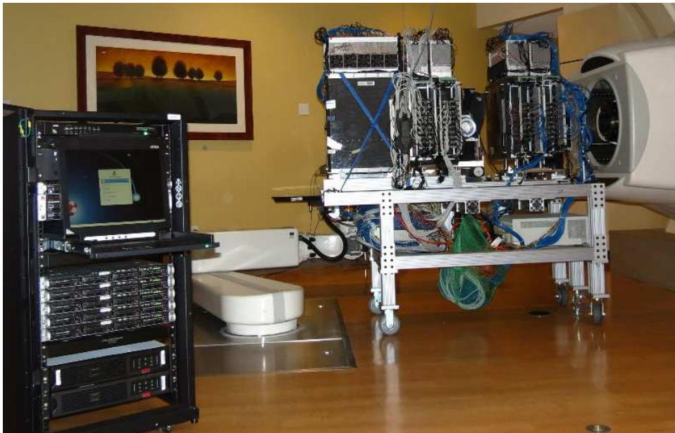
Figure 3: Fully assembled DAQ cluster system (left) and proton CT scanner (right) at CDH Proton center. From right to left, beam enters upstream tracker planes followed by downstream tracker planes and finally the calorimeter. The gap in the middle is where the rotation stage for rotating the head phantom in the horizontal plane is placed.
