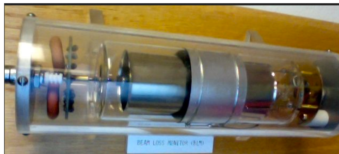
Visualisation of ion chamber operation
