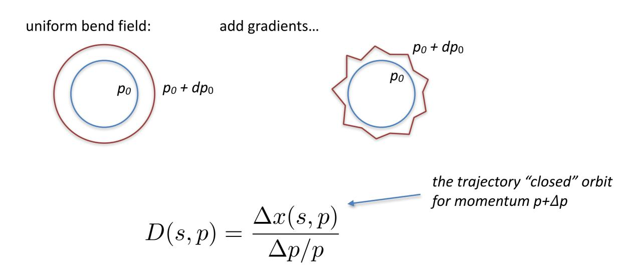
the orbit of an off-momentum particle which closes on itself is described by the *periodic* dispersion function
