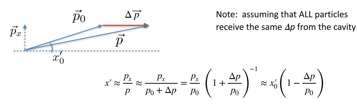
Note: particles at peak of their betatron oscillation will have little/no change in x', while particles with large transverse angles will have their x' affected most
