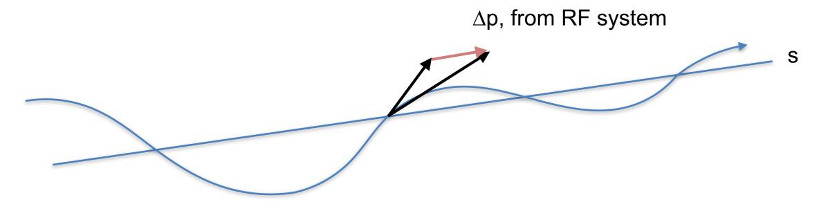
The coordinates x-x' are not canonical conjugates, but x-px are; thus, from classical mechanics, the area of a trajectory in x-px phase space is invariant for adiabatic changes to the system.
