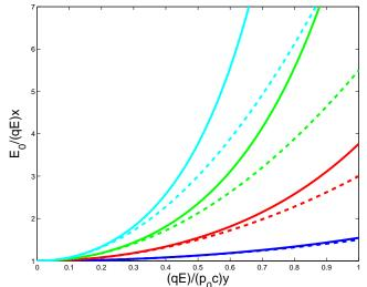
Trajectories (in normalized coordinate) in uniform constant E-field:  $\hat{x} = \cosh(\kappa \hat{y})$ , with  $\kappa = 1, 2, 3, 4$ . dashed are corresponding parabolic approximation  $\hat{x} = 1 + \frac{1}{2}(\kappa \hat{y})^2$ .
