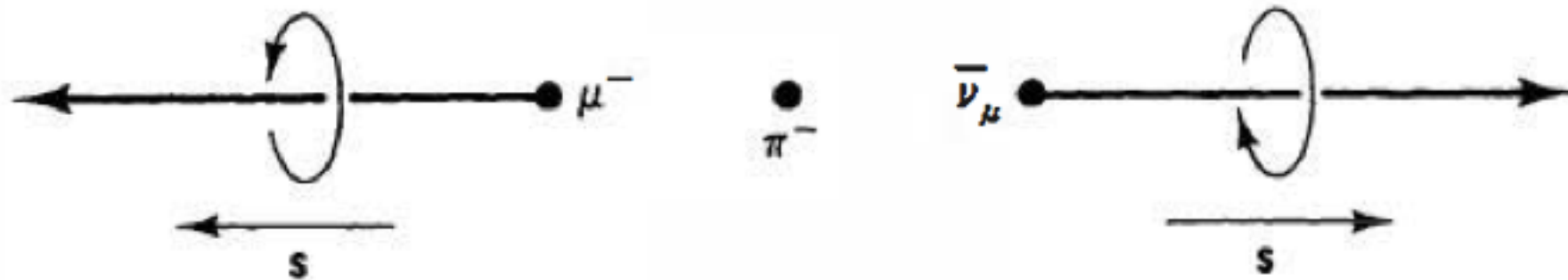
Fig. 4.10 Decay of \pi^- at rest.
