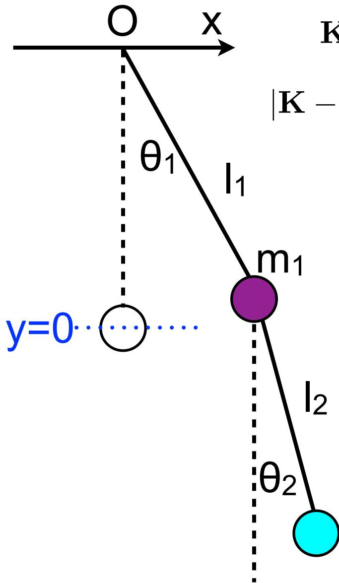
$$\mathbf{K} - \omega^2 \mathbf{M} = ml^2 \begin{bmatrix} 2\omega_0^2 - 2\omega^2 & -\omega^2 \\ -\omega^2 & \omega_0^2 - \omega^2 \end{bmatrix}$$
