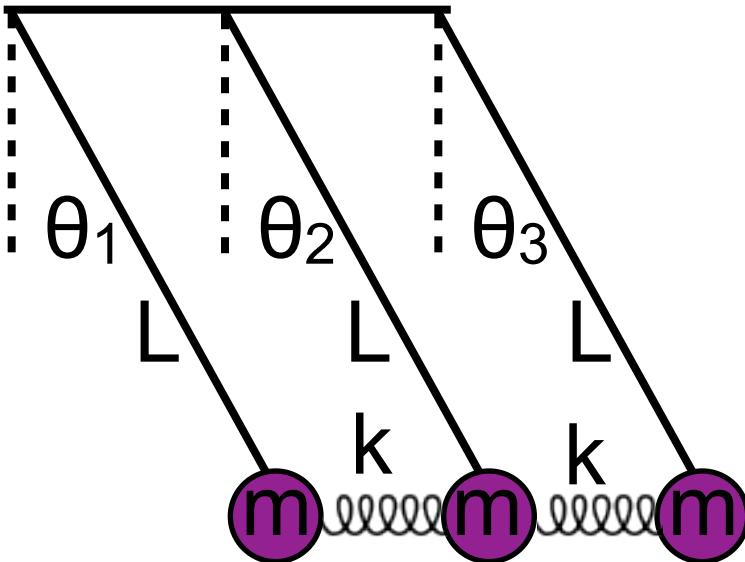
To first order, pendulums don't move in y direction, only x direction, and change is  $I \sin(\theta) \sim I\theta$ . So ...
