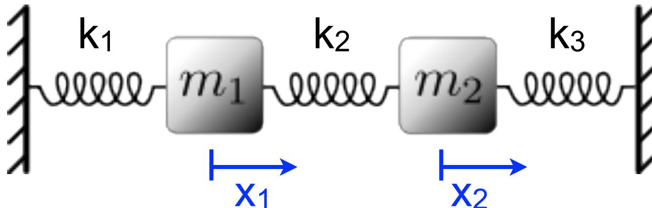
So in first normal mode both blocks move together, as if  $k_2 = 0$ , with frequency  $\omega = \sqrt{k/m}$
