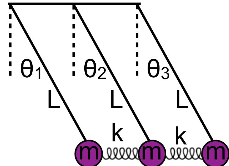
Three equal mass attached via pendulums of equal length, connected via two springs of the same spring constant. What is the motion?
