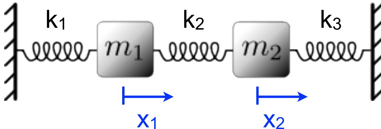
If  $k_2 = 0$  then springs are not coupled to each other, but with  $k_2$  can see that if  $m_1$  moves to the right, then this compresses  $k_2$  and will push  $m_2$  to the right (for example)
