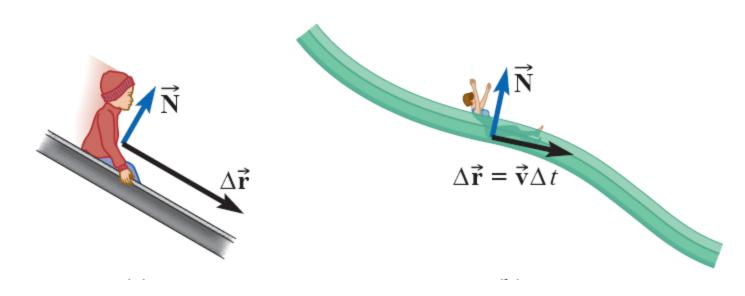
The normal force does no work when it is perpendicular to the displacement.
