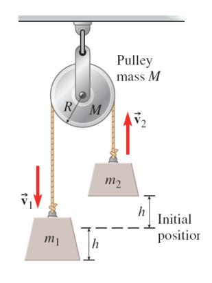
If the masses are released from rest, find how fast they are moving after they have moved a distance *h* (one up, the other down).
