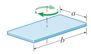
Perpendicular  $\frac{1}{12}M(a^2 + b^2)$  to plate through center
