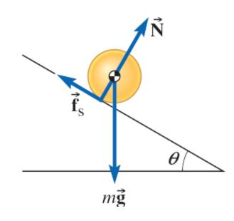
The frictional force  $\vec{f}$  provides a torque  $\tau = rf$
