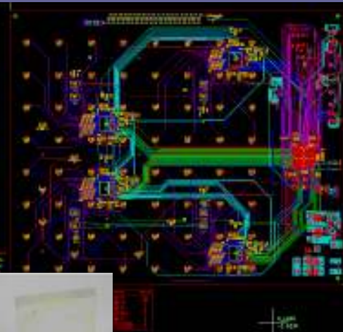
Previous tile design w/ WLS Fiber optic & SiPM
