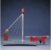
The ratchet does not directly measure the height, but is marked off in arbitrary units that go from 0 to 40 in steps of 10. There are marks at the halfway points (5, 15, 25, 35), and each individual ratchet position that represent steps of 1 unit. The height displacement has been measured for the labeled positions and can be found in Table 1.
