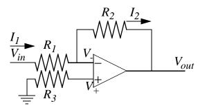
• The bias current is pulled into the inverting input through both  $R_1$  and  $R_2$ . If  $R_3$  is equal to the parallel equivalent of  $R_1$  and  $R_2$  the voltage drops will cancel.
