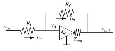
• The output impedance is:  $Z'_{out} = v_{th} / i_s$ .
