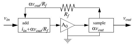
If the input impedance for the amplifier  $A_0$  is very large, no current can flow into the amplifier • compared to the input and feedback, so the input must cancel the feedback.  $i_{in} = \frac{\alpha v_{out}}{R_f}$
