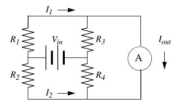
• If the current meter shows  $I_{out} = 0$ , there are two balance equations.
