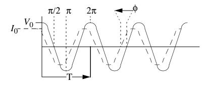
• The RMS voltage and current,  $V_{\rm rms}$ ,  $I_{\rm rms}$ , are related to the amplitude.
