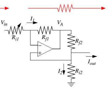
• The variable resistor can be adjusted until the resistors meet the following ratio:  $\frac{R_{f2}}{R_{f1}} = \frac{R_{i2}}{R_{i1}}$
