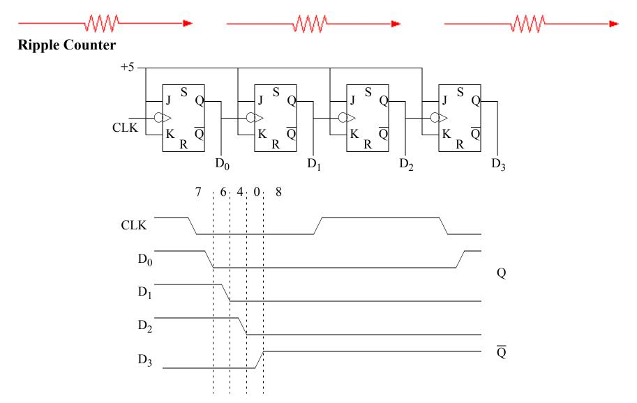
In a ripple counter at a clock edge each data bit much change before the next higher bit can change. The apparent counts that exist during the clock transition are called *transients*.
