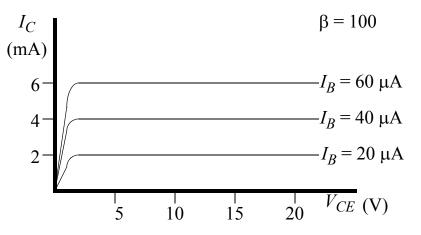
In the above example, as  $I_B$  goes from 20  $\mu$ A to 60  $\mu$ A, I<sub>C</sub> goes from 2 mA to 6 mA. The ratio 4 mA / 40  $\mu$ A = 100 =  $\beta$ .
