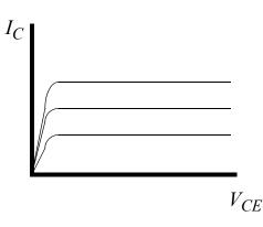
• Selecting  $V_{BE}$  and  $V_{CE}$  determines the behavior of the transistor LABORATORY ELECTRONICS I
