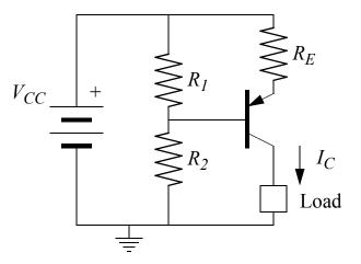
• With the pnp the load can be directly attached to ground if the power supply is positive.
