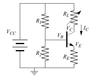
$V_C = V_{CC} - I_C R_L$  $V_B = \frac{R_2}{R_1 + R_2} V_{CC}$
