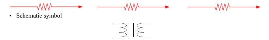
Transformers are a pair of inductors around a common center used to convert AC voltages to lower or higher values.
