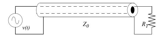
• If the circuit is open, the reflected wave bounces back along the center conductor with the same magnitude as the incident wave arrived.
