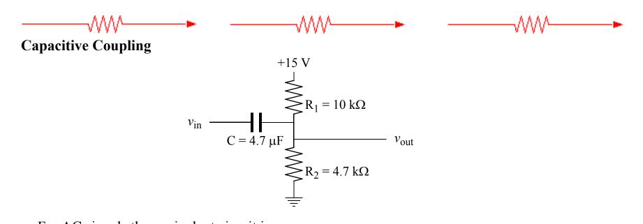
• For AC signals the equivalent circuit is
