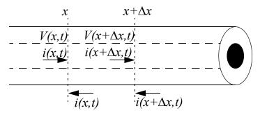
The voltage and current are both functions of position and time
