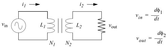
Magnetic flux in the the primary coil is carried into the secondary coil. Induced current depends on the magnetic flux in the secondary coil
