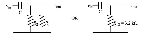
• The high pass breakpoint is at  $f = 1/2\pi R_{12}C = 10.6$  Hz.
