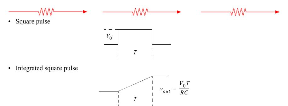
• The peak of the integrated pulse is proportional to the area of the initial pulse.
