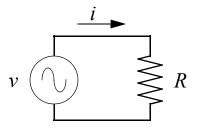
• For an AC voltage through a resistor current and voltage have the same phase.  $\phi = 0$ ,  $\cos\phi = 1$ .  $P = V_0 I_0 / 2 = V_{\text{rms}} I_{\text{rms}}$ .
