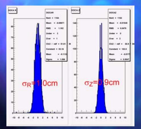
Impact parameter and momentum resolution must improve when the tracks link to hits in outer layer of tracking device.
