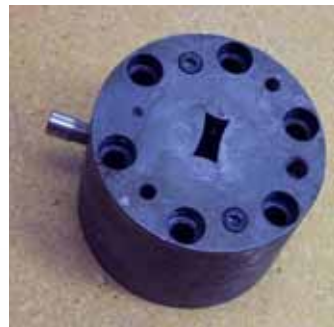
2x1cm rect. die developed at NIU for Lab 5
