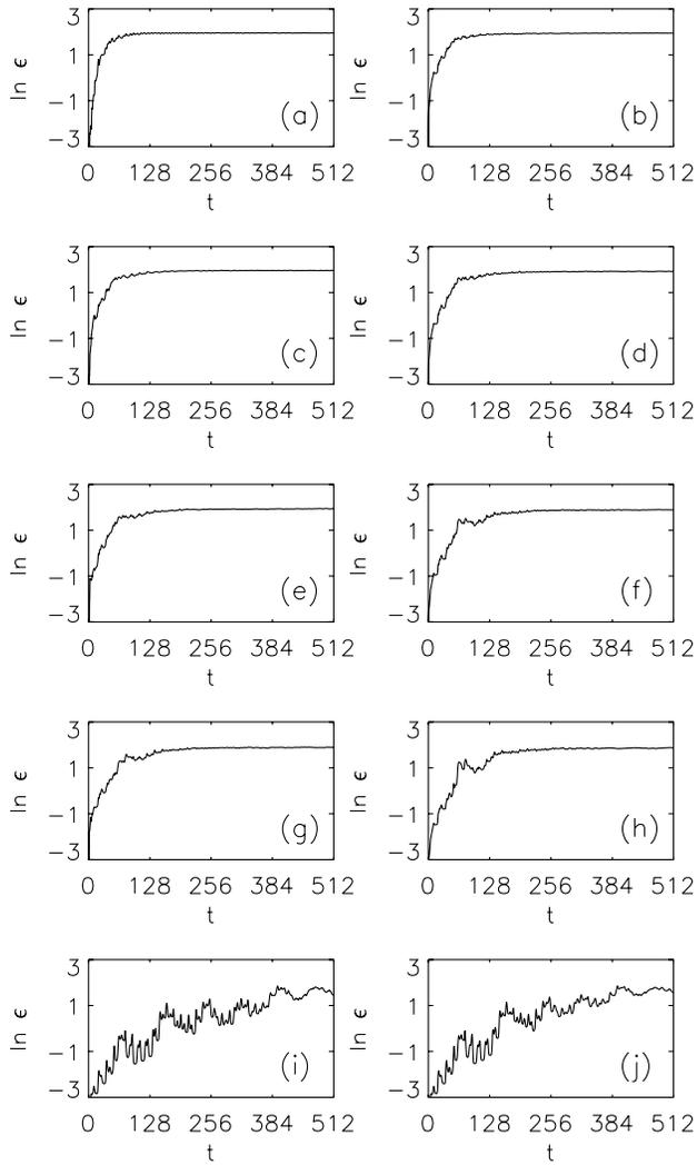
FIG. 6. Same as Fig. 5 but for a clump of chaotic orbits. (a)  $N = 10^{4.5}$ . (b)  $\eta = 10^{-3.0}$ . (c)  $N = 10^{5.0}$ . (d)  $\eta = 10^{-3.5}$ . (e)  $N = 10^{5.5}$ . (f)  $\eta = 10^{-4.0}$ . (g)  $N = 10^{6.0}$ . (h)  $\eta = 10^{-4.5}$ . (i) Unperturbed motion in the smooth potential. (j)  $\eta = 10^{-8.0}$ , the largest noise amplitude that does not appreciably alter the results generated in the smooth potential.
