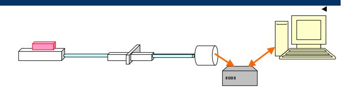
Cell with WLS fiber irradiated by a radioactive or LED WLS fiber connected to clear fiber which is connected to a photo detector (PMT's, VLPC's etc.)
