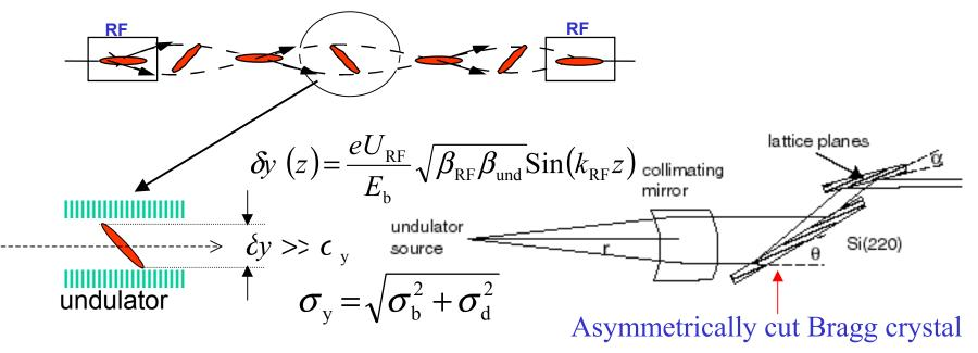
Diffraction limited size of a source at  $\lambda \neg 1$ Å:  $c_d \sim 3 \mu m$ Beam size at  $\epsilon_n = 0.4 \text{ mm-mrad}$ :  $c_b \sim 14 \mu m$
