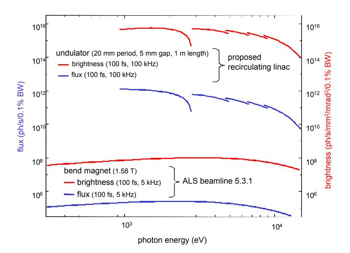
Average femtosecond flux and brightness compared with that of the existing bend-magnet fs beamline.
