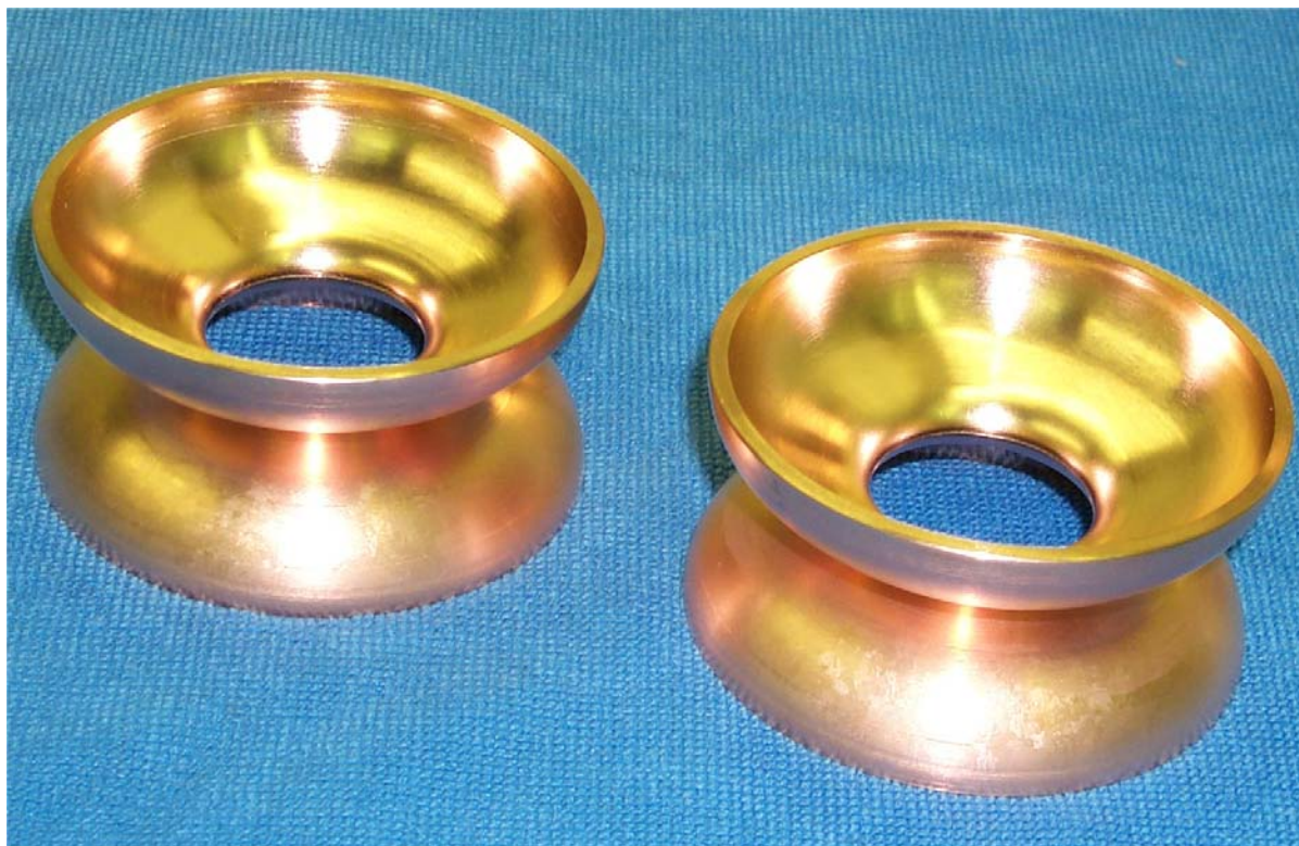
Two dumbbells brazed in vacuum furnace ( 65\text{Cu}/35\text{Au} )
