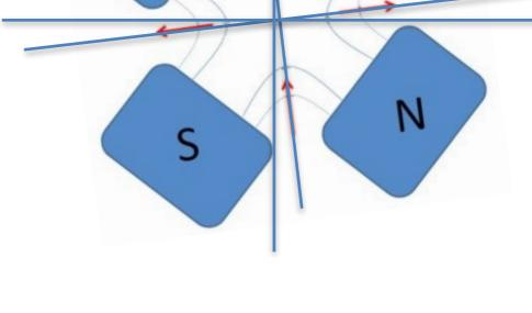
Clearly, skew quad field couples the horizontal and vertical motion:
