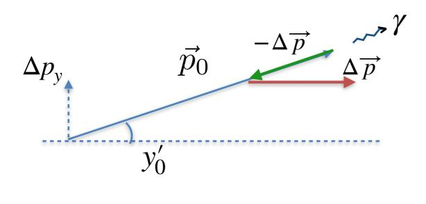
The particle will lose energy due to the emission of photons, but the energy will be replenished by the RF system in the ring.
