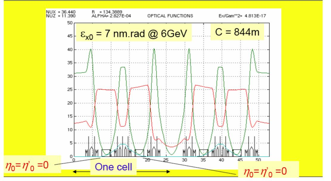
Original lattice of ESRF storage ring, with 4 quadrupoles in between the bends
