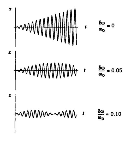
ex: transverse wake fields driven by average offsets of the particles
