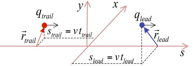
$$V_W(\vec{r}_{lead}, \vec{r}_{trail}, t_{trail} - t_{lead}) = \int_{-\infty}^{\infty} \vec{E}_W(s, \vec{r}_{lead}, \vec{r}_{trail}, t_{trail} - t_{lead}) \cdot d\vec{s}$$
