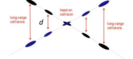
crossing angle,  $\theta$   $d \sim \theta L$ and want  $d \sim n\sigma = n\sigma^* (\beta/\beta^*)^{1/2}$
