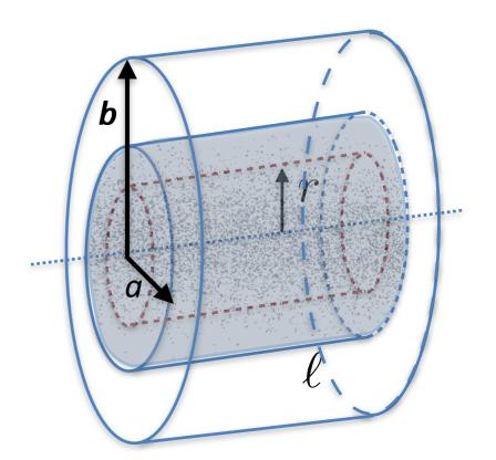
$$E_{r} = \frac{\lambda}{2\pi\epsilon_{0}} \frac{1}{r}, \quad B_{\phi} = \frac{\mu_{0}\lambda v}{2\pi} \frac{1}{r}, \quad r \ge a; \qquad \oint \vec{E} \cdot d\vec{\ell} = -\frac{\partial}{\partial t} \int \vec{B} \cdot d\vec{A}$$
